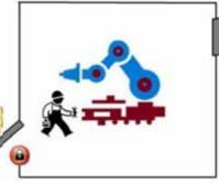
from different locations or troubleshooting different parts of the machine simultaneously. However, when multiple switches are activated, the activation of each switch resets the previous switch. Therefore, if there is a fault in the first switch, activating the second switch "masks" it.
