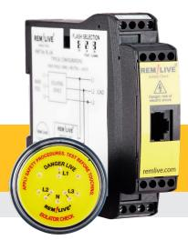
The **REMLIVE RL-24i** Isolator Check provides the user with a positive check when isolating plant. It provides electrical isolation between the DIN rail unit and the door mounted display unit. The door unit is designed to fit through the front of a control panel or switch so the user can see a live/isolation status. The super bright REMLIVE RL-24i display provides the user with a quick and easy method of proof of isolation in lock out / tag out procedures.
