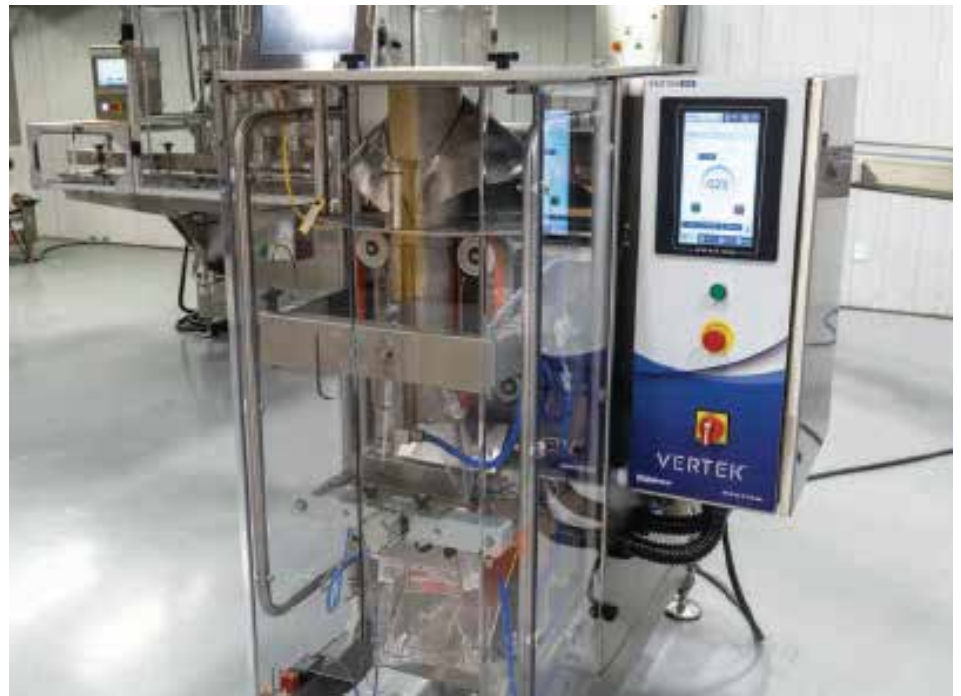
Omron servo drives and inverters ensure precise motion control and product positioning at exceptionally high operating speeds of up to 200 packages per minute.
