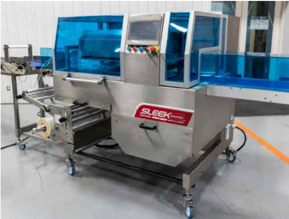
Manufactured by Paxiom, the SleekWrapper ValTara series automatic flow wrapping machine above incorporates advanced Omron servo drives and inverters (bottom left) to ensure precise motion control and product positioning at exceptionally high operating speeds of up to 200 packages per minute.
