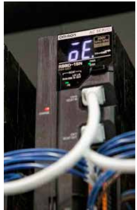
Omron's AC Servo Series with built-in EtherCAT communications.
