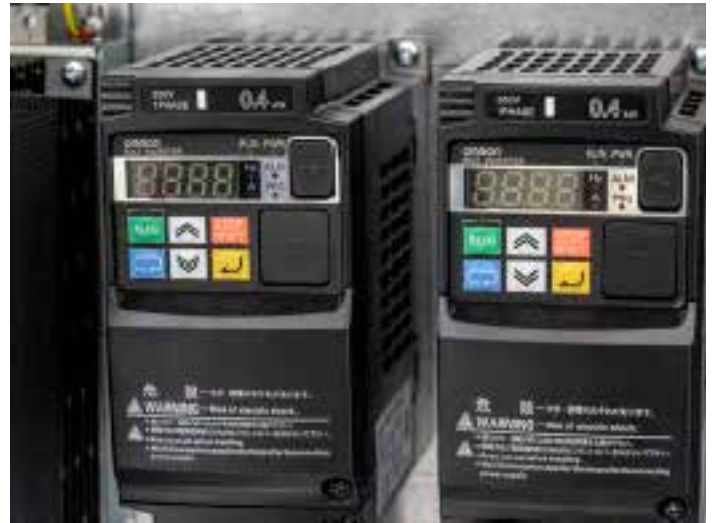
Omron servo drives and inverters ensure precise motion control and product positioning at exceptionally high operating speeds of up to 200 packages per minute.
