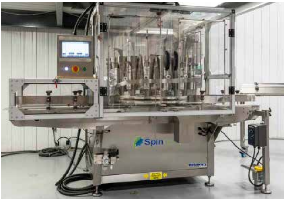
Also manufactured by WeighPack, the SpinDexer container filling machine on the right incorporates Omron's Sysmac CP1H PLCs (programmable logic controllers) shown in the pictures below to fill up to 60 to 70 bottles per minute with various types of dry and powder products.
